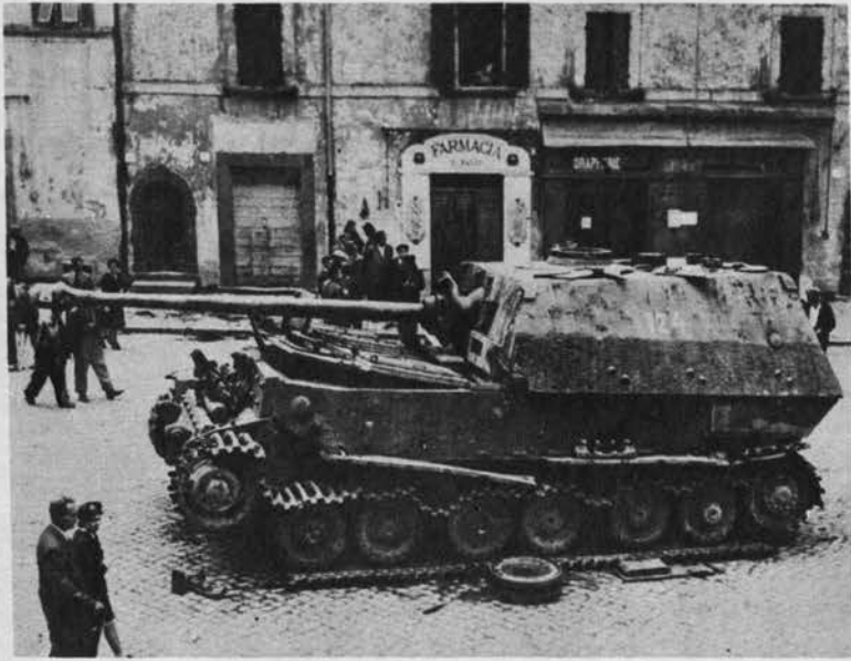
Ferdinand , Nazi 72-ton heavyweight, has 88-mm. gun and 8-in. armor on its bow. Picture shows one of the captured 12½-m.p.h. vehicles.
